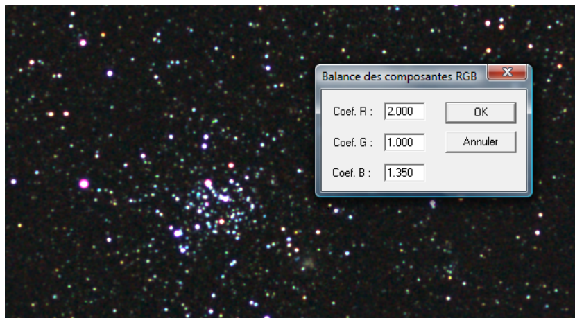
FIG. 13 – One of RAW image before any processing. The green color is typical of an unprocessed RAW file. It means that the sensor used is manifestly more sensitive in the green channel compared to the red or blue channels. Note the presence of optical vignetting.
