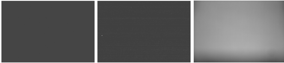
FIG. 7 – From left to right, the image OFFSET, image DARK, image FLAT85.
