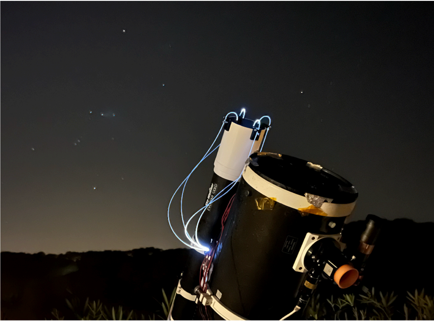
Use of economical optical fibers (plastic) for precision spectral calibration at the entrance pupil.
