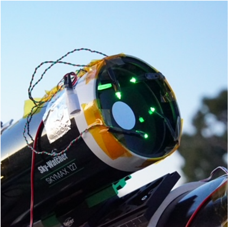
Example of spectral calibration setup on the pupil
