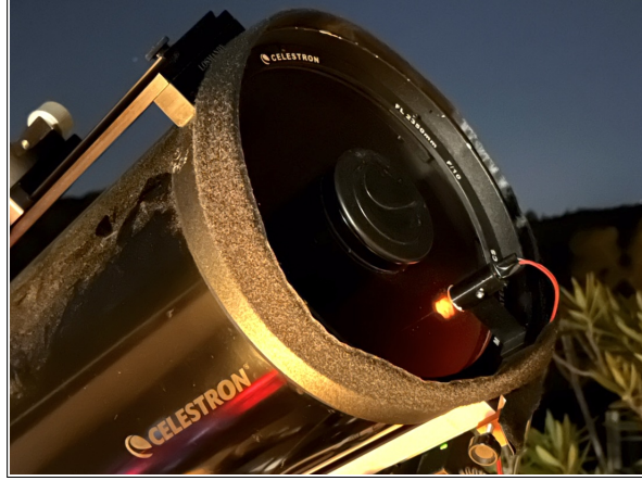
Figure 92 – Another approach is to place the calibration lamp directly in front of the pupil, without using a fibre (the telescope here is a Celestron C9.25).
