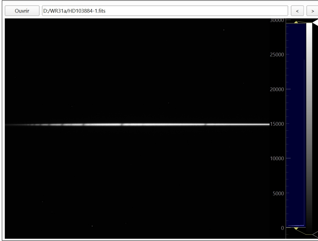
Figure 120 – Detail of one of the images of the star HD 103883 (blue part of the spectrum). The Balmer lines appear as fine notches cut into the spectral continuum.
