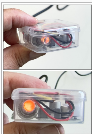
Figure 139 – The wavelength-calibration lamp, ready for use.
