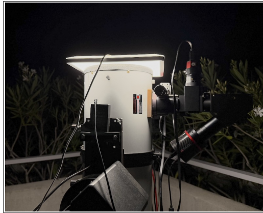
Figure 31 – Exposure of the spectrum of the flat lamp (an LED panel).
