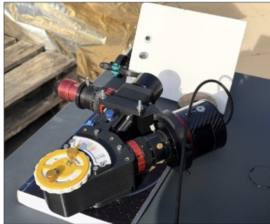
Figure 83 – Measuring the calibration parameters of a spectrograph, here a Star’Ex LR.
