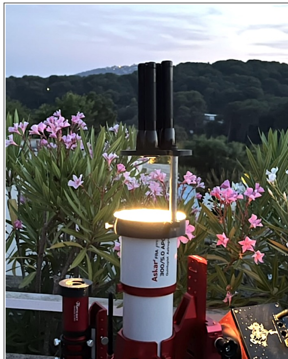
Figure 99 – Acquiring a flat-field using torches fitted with tungsten-filament bulbs (MagLite brand — take care not to use LED models). A diffuser (a sheet of tracing paper) should cover the entrance of the refractor. Recall that, within the processing scheme presented in this guide, obtaining such a flat-field (called “PLU” in French, for Plage de Lumière Uniforme , i.e. a uniform-illumination field) remains optional, not compulsory. The purpose of this flat-field is essentially to smooth out pixel-to-pixel sensitivity differences (PRNU = Pixel Response Non-Uniformity ), which are very slight with modern sensors.
