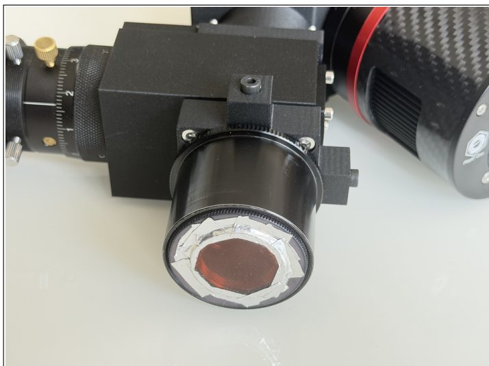
Figure 136 – Improvised fitting of an order filter at the front of a TSE spectrograph in order to take spectral images in the infrared.
