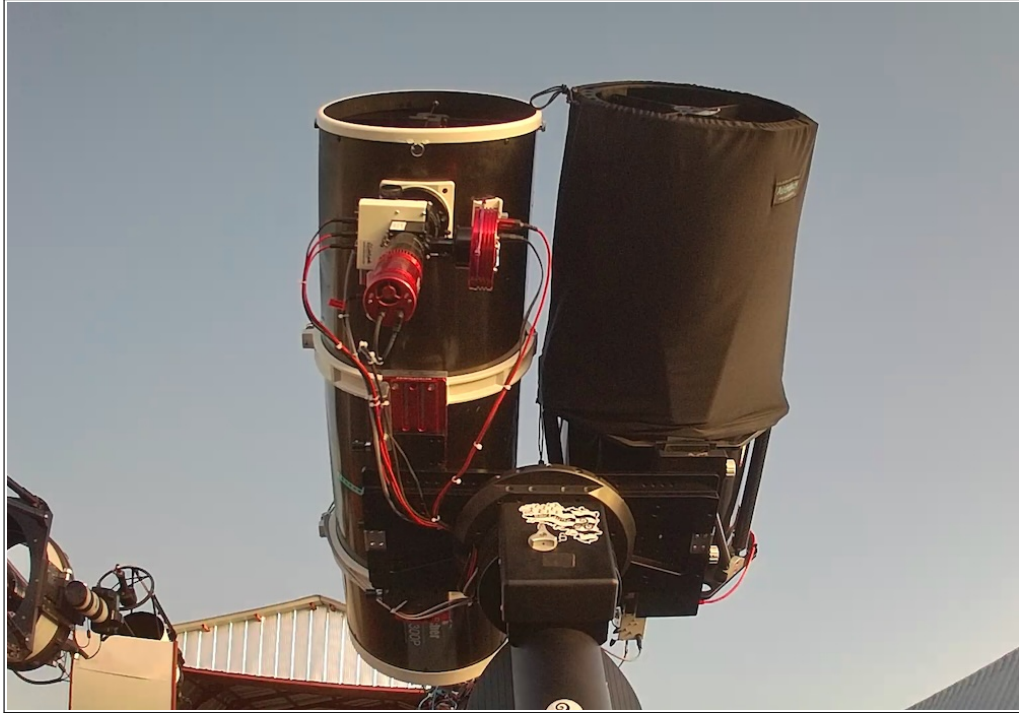
Figure 118 – The equipment located in Chile and operated from France by the 2SPOT team. The optical tube of interest here is the one on the left: a 305 mm f/4 Newtonian telescope with the Alpy 600 spectrograph at the focus.
