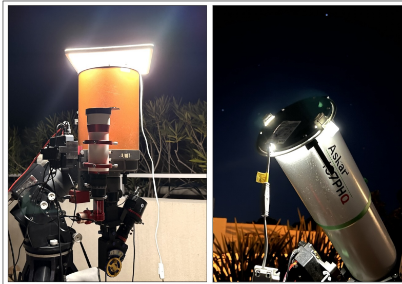
Figure 88 – Acquiring a flat-field using a household LED lighting panel. Although the LED spectrum is not very uniform across the whole visible range, using one remains sensible for calibrating high-resolution spectra around H\alpha . The image on the right shows the setup mounted in front of the Askar 107PHQ refractor; on the left, in front of a venerable orange Celestron 8.
