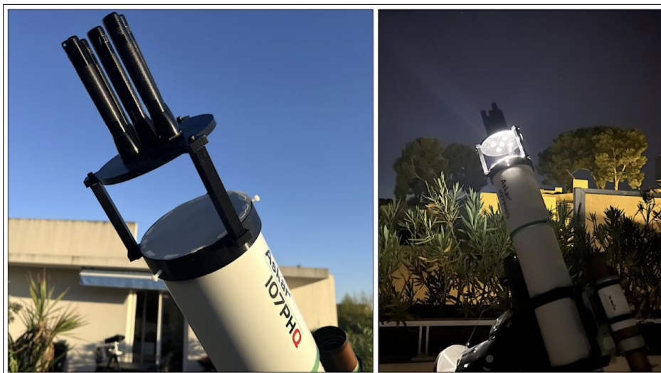
Figure 104 – Setup used to acquire the low-resolution flat-field, using incandescent-filament lamps producing a “black-body”-type spectrum.
