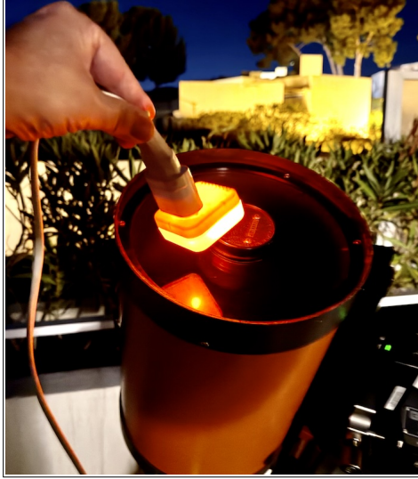
Figure 69 – A neon night-light waved in front of the telescope aperture to obtain a spectrum of wavelength-calibration lines in an image separate from the one being calibrated (a stellar spectrum, typically).
