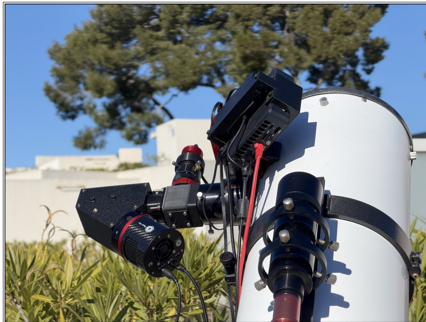
Figure 2 – The TinyStar’Ex spectrograph mounted at the focus of a 200-mm Newtonian telescope.
