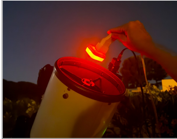
Figure 30 – Exposure of the spectrum of the reference spectral lamp (a neon night-light).
