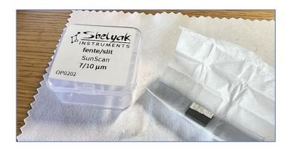
Occasionally, an incident may require cleaning both sides of the glass plate. Although the coatings on these sides are relatively durable, it's essential to remember that these are optical components, requiring special care. Avoid rubbing them with paper or a used cloth, and do not use standard cleaning products, especially those meant for household windows.
