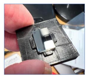
As a last resort, you can try to blow away residual dust or cotton fibers using a can of compressed air. Be careful, as it is very important to follow a few rules when using this type of compressed air canister: (1) purge with one or two short bursts to remove impurities before approaching the slit, and (2) blow with the nozzle always held horizontally and the canister in a vertical position; this is crucial to avoid propelling anything other than dry air onto the glass surface.
