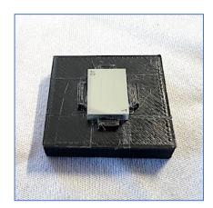
It is important to identify the relevant glass face, specifically the one coated with chrome. As a reminder, in the Sol'Ex, the chrome-coated side of the slit (where the slit is photolithographed, meaning the exact plane of the slit) faces outward, causing the inscriptions to appear upside down once installed.
