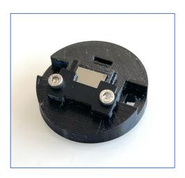
The Sol'Ex GEN2 slit installed in the Sol'Ex instrument:
