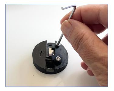
GEN2 slit mounted in its holder. For use with Sol'Ex, we recommend turning the slit so that the chrome-plated side faces outwards (the letters indicating slit widths are then read in reverse):
