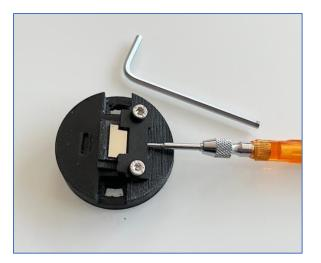
There's no need to tighten the two M3 flange retaining screws:
