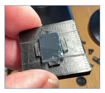
The most problematic dust particles are those on the chrome-coated side, as they produce fine transversalium traces, which are more difficult to remove during data processing.
