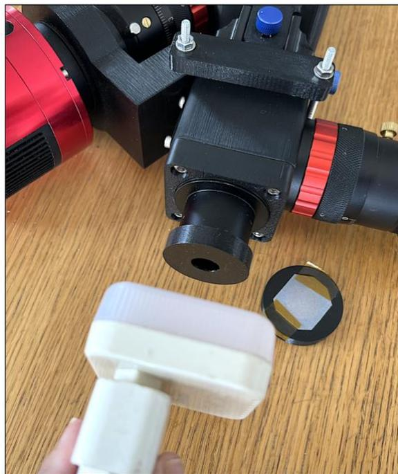
*Figure 6. Illumination of the Star'Ex entrance with a neon source.*
