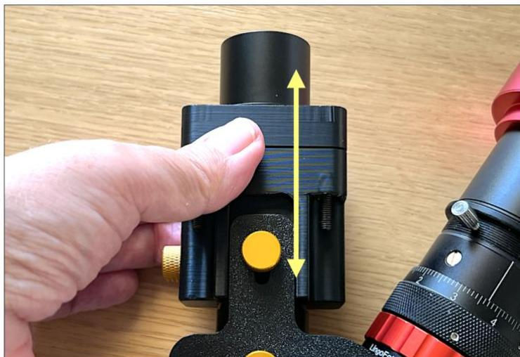
Figure 12. The adjustment of the distance from the slit to the collimator.
