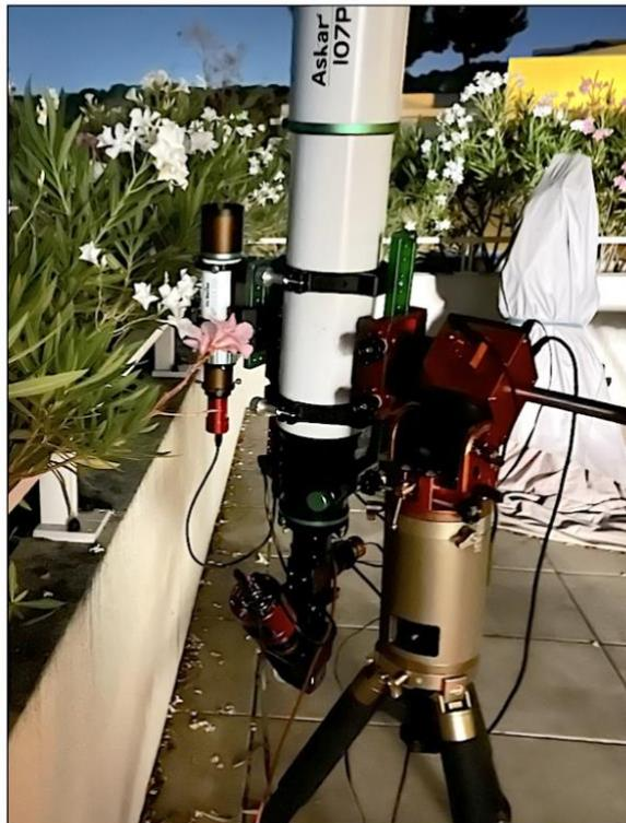
*Figure 22. Askar 107PHQ telescope to which Star'Ex is attached, all mounted on a ZWO AM5 mount.*
