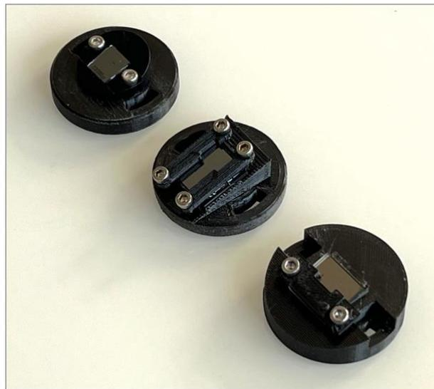
*Figure 1. A set of slits compatible with Star'Ex. On the left, a slit initially designed for the Alpy600 spectrograph. In the center, an arrangement with four slits of varying widths, originally used with the Lhires III and LISA spectrographs from Shelyak. On the right, the new Star'Ex GEN2 slit in its 3D-printed holder.*
