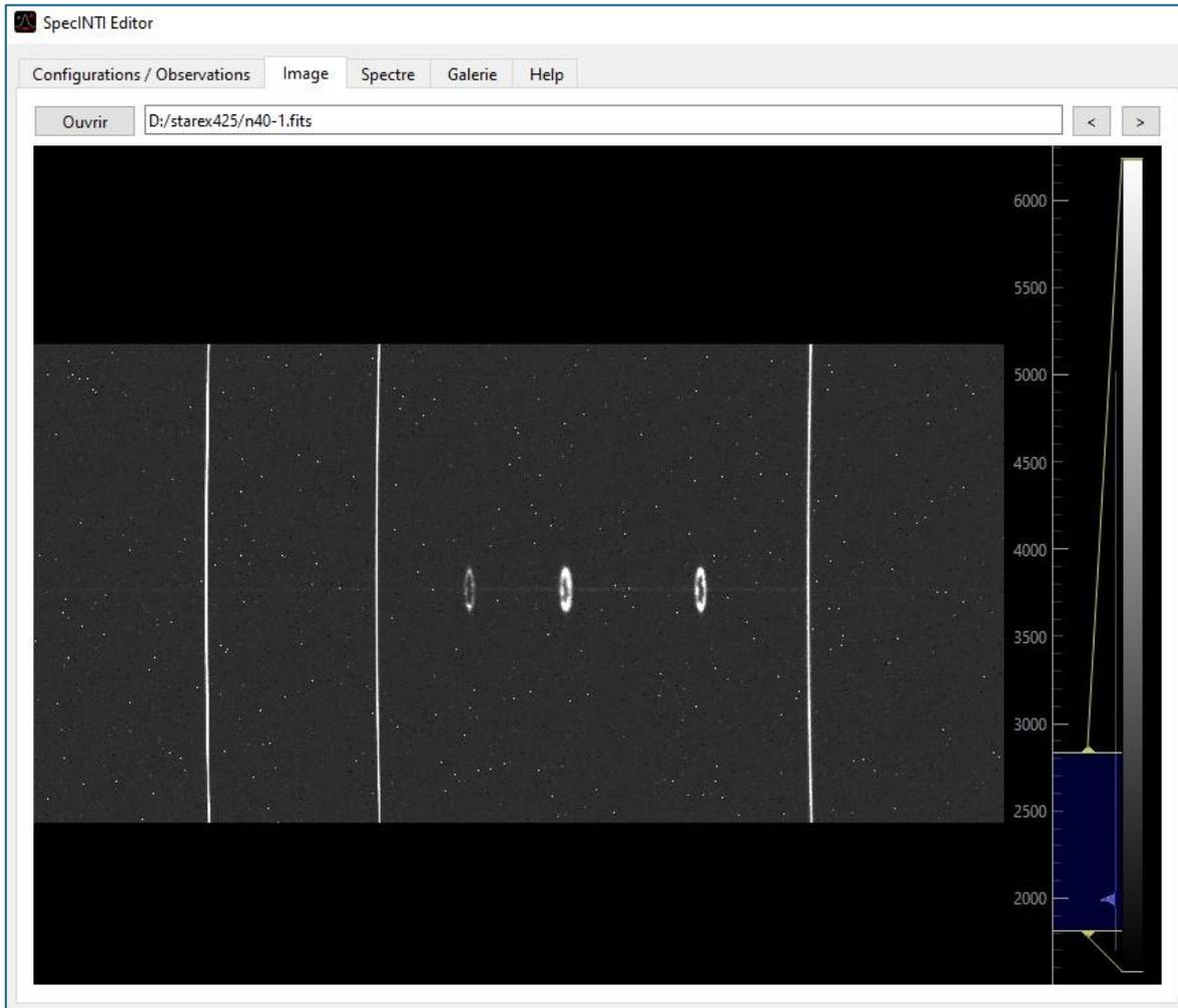
The oval shape of the lines (hydrogen + nitrogen) is due to the radial expansion velocity of the gas in the nebula (Doppler-Fizeau effect).
