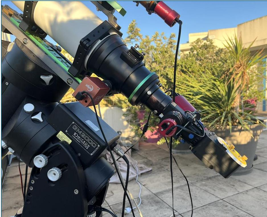
The center of the telescope's entrance pupil is illuminated continuously by a 1 mm-diameter plastic optical fiber, connected to a neon lamp at the other end. We therefore work in **lateral mode**: the line spectrum of the neon lamp is recorded simultaneously with that of the star. We focus on a region of the spectrum covering the H-alpha line (6563 Å) and the red He I line (6678 Å).
