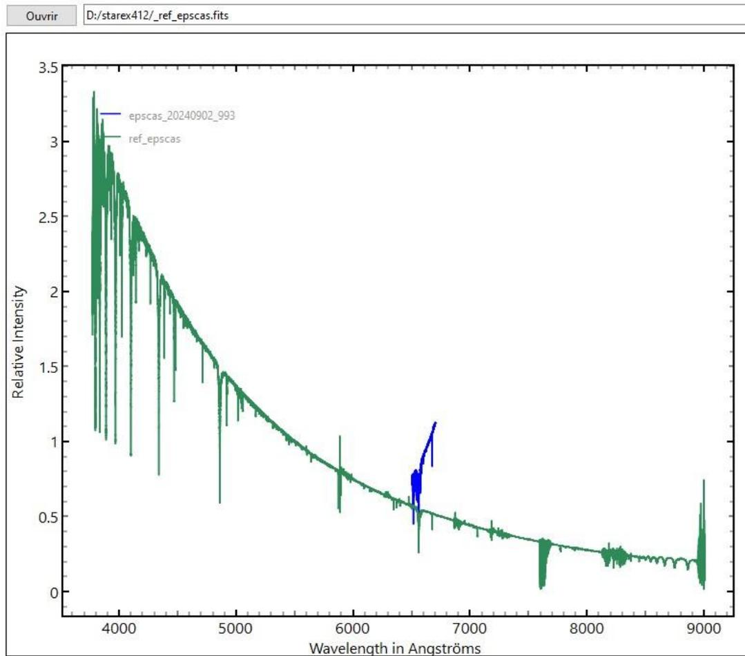
The Star'Ex spectrum is displayed in blue. It covers only a small portion of the visible spectrum. Enlarge the area around the H-alpha line:
